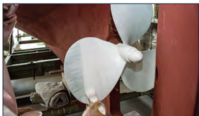
Applying second coat of Velox Plus Paint.
