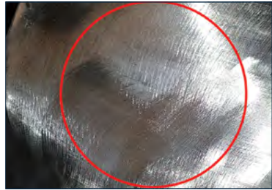
Red circle showing same prop sanded thoroughly using 80 grit sand paper.
