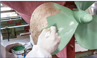
Applying Metal Primer.
