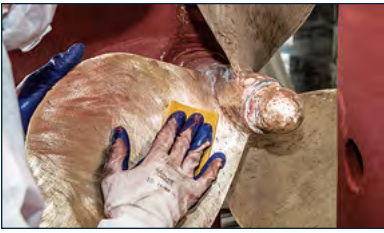
Aggressively sanding hard to reach spots with 80 grit sand paper.
